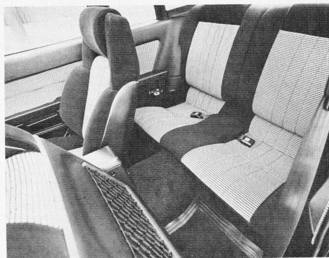
Unusual for a notchback: rear seatbacks fold separately for trunk access.
